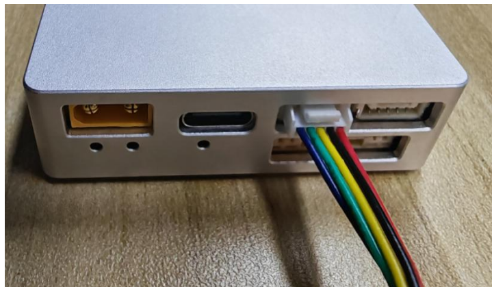
Figure 1-8 RS422 connection method
